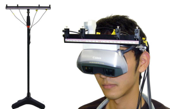
Figure 2: Microphone arrays (Left: fixed type, Right: wearable type)
