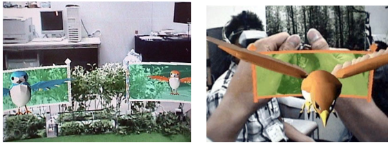
Figure 3: Users can select a menu item using a sound direction. In this figure, a birdcall is used as a sound device.
