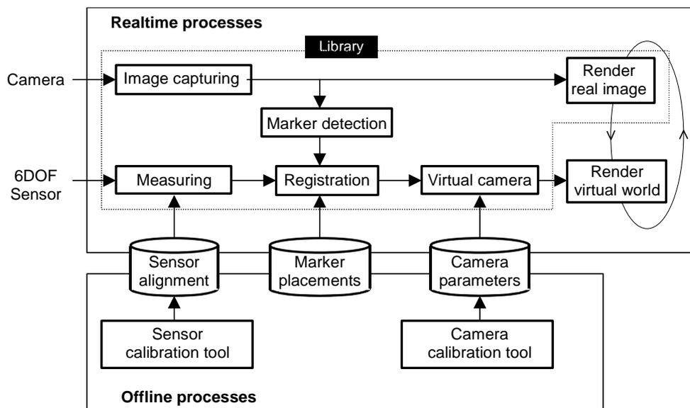
Figure 11: Processing elements of MR Platform system.
