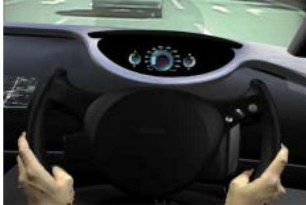
Figure 8: Composition of real scene, virtual instruments, and real hands.
