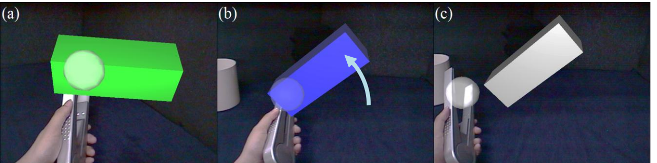
Fig. 8 TweezersDevice operation. (a) Pick (b) Move (c) Release
