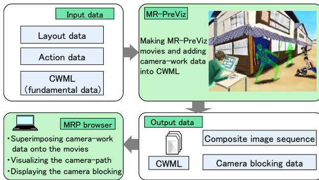
Figure1. The flow diagram of camera-work authoring tools
