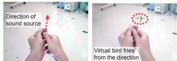
(b) When the user generates a sound with the birdcall, the virtual bird selected in Figure 5 (a) flies from the direction to him/her.
