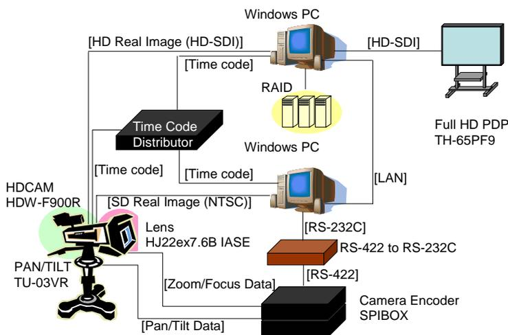
**Figure 3 System configuration**
