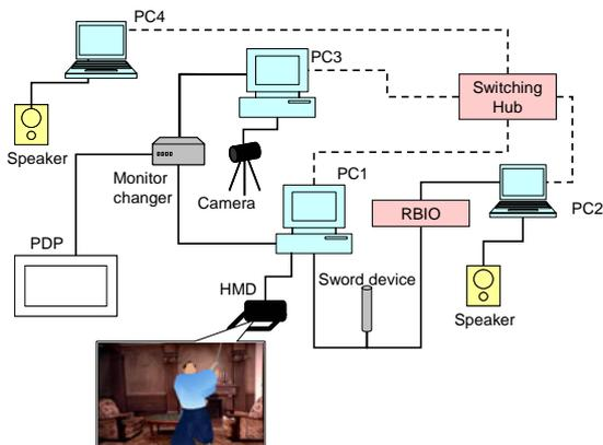
**Figure 9** System configuration of MR-based action rehearsal system
