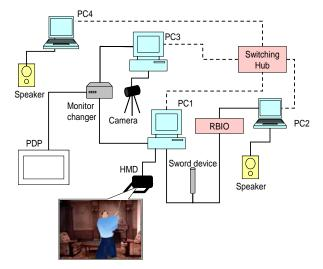
Fig. 9. System configuration of MR action rehearsal system.
