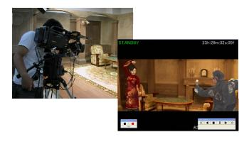
Fig. 2. Aspect of MR-PreViz image capturing and compositing system. (Left: Appearance, Right: Screenshot of composite images)
