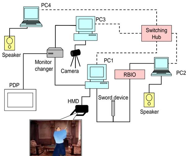
Fig. 9. System configuration of MR action rehearsal system.
