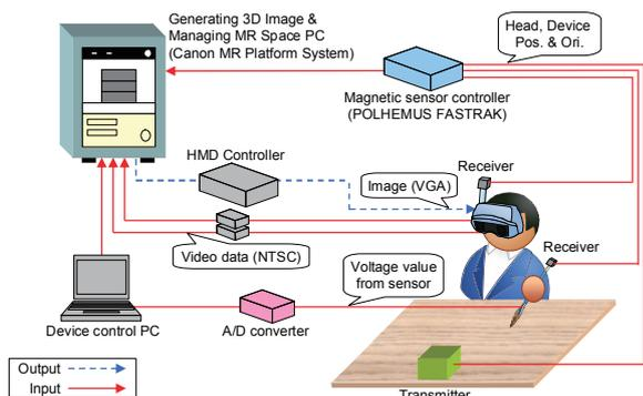
Fig. 5 System configuration
