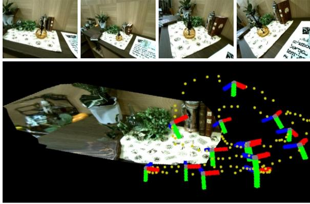
Figure 5: Visualization of camera poses estimated using tracking by the synthesis-based [26] approach. The top row shows several frames used for this tracking. The bottom figure shows plots of camera pose and a tracked T-3DM. Note that the undesirable object is not included in the T-3DM.
