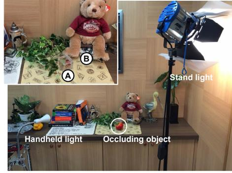
Figure 11: Indoor test scene. Lighting is changed using the stand light with a diffuser sheet and the handheld light.
