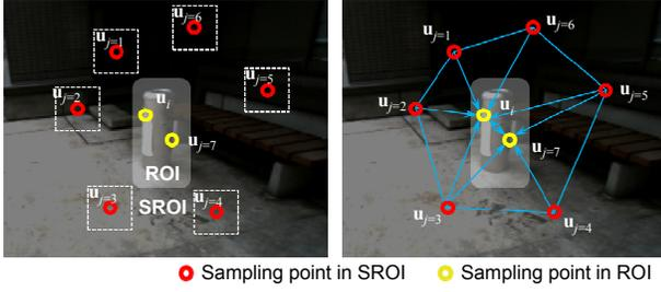
Figure 8: Color ratio measurement in SROI (Left) and color ratio estimation in ROI (Right). In this figure,  $u_i$  is estimated using  $u_1, u_2, u_3, u_7, u_5,$  and  $u_6$ .
