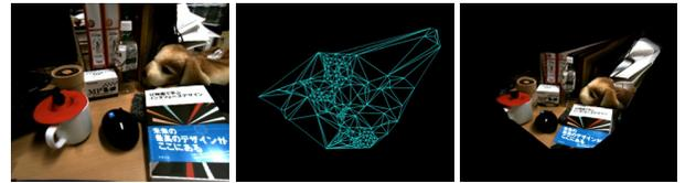
Figure 4: Examples of T-3DM. From left to right, real scene: geometry proxy (3D polygon meshes), and IBR rendering result.
