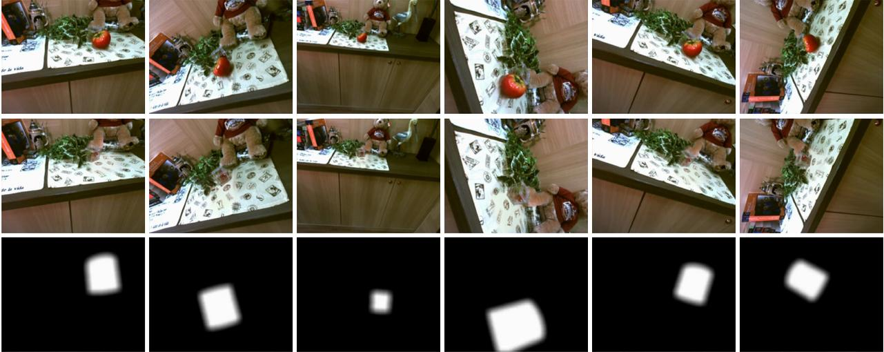
Figure 12: Pairs of original frames, corresponding DR results, and mask images for the indoor test scene. Illumination was varied (from the first row to the other rows) after pre-observation.
