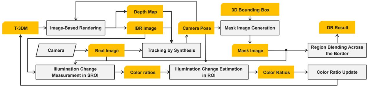
Figure 3: Data flow of the proposed method. Note that it recycles IBR image and corresponding depth map (z-buffer) both for a geometric and photometric registration.
