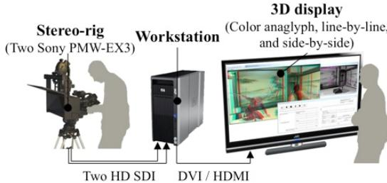
**Fig. 3.** System configuration
