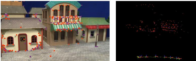
**Fig. 4.** Examples of tracking result. Left: Map reprojection. Three maps are reconstructed and each of them is colored just for visibility. Right: Bird's eye view of the 3D reconstruction and camera trajectory.
