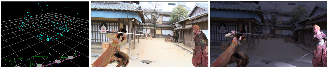
Figure 1: Our method (left: Structure-from-motion, middle: Match move, right: Relighting)
