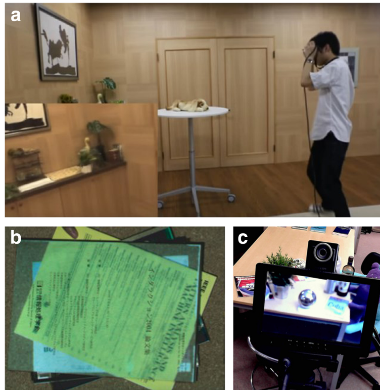
Fig. 3 See-through-based, projection-based, and tablet-based DR systems. This figure shows see-through-based [103] (a), projection-based [82] (b), and tablet-based [35] (c) DR systems
