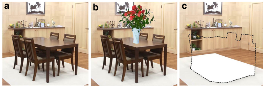
Fig. 1 Real, augmented, and diminished scenes. This figure shows differences between real (a), augmented reality (b), and diminished reality scenes (c). In augmented reality, real–virtual inconsistency mainly appears where real and virtual objects contact each other, i.e., geometric registration of virtual objects is one of the most important issues. From this point of view, in DR, real–virtual borders will appear all around the virtual regions since real regions surround the virtual ones
