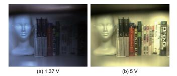
Figure 9: Turbidity (a) and non-uniformity (b) of the used LCD shutter.
