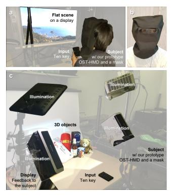
Figure 4: Experimental setups of our psychophysical study. (a) Experimental setup in Scene 1 for flat environment in a black box. (b) A subject with our prototype OST-HMD and a mask to shut off external lights. This fully covered mask is simply for complete avoidance of external lights and therefore could be replaced with commodity masks, such as covers for video see-through HMDs. (c) Experimental setup in Scenes 2 and 3 for the 3D environment.
