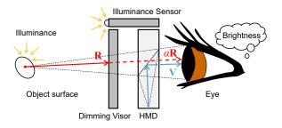
Figure 2: Schematic figure of the proposed OST-HMDs with dimming visors. The user receives the real light *R* through the unit angle  $\omega$ . While the virtual light *V* is directly projected to the eye by a display of HMD, the real light *R* is dimmed by the dimming visors to  $\alpha R$ .
