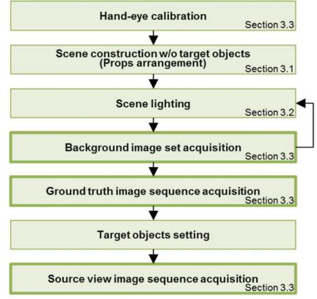
**Fig. 8** Basic workflow of the proposed data acquisition method (boxes with heavy lines are the three phases in Fig. 1 and boxes with thin lines are preparation phases).
