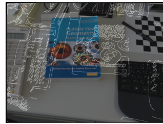
Figure 3: Interactive relocalization. Edges detected in a keyframe image for relocalization are overlaid onto a camera image.
