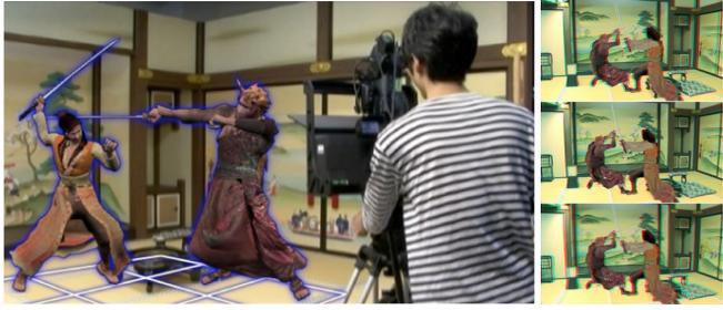
**Fig. 2.** Image of on-set S3D MR-PreViz. Left: CG-animated characters are superimposed in realtime and it enables stereographers to confirm the results in the early stage. Right: Results of disparity adjustment in S3D MR-PreViz system.
