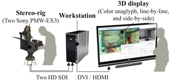
Fig. 3. System configuration
