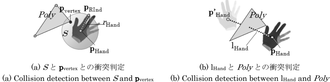
図8 「叩く」ジェスチャの衝突判定 Figure 8: Collision detection of "slapping" gesture
