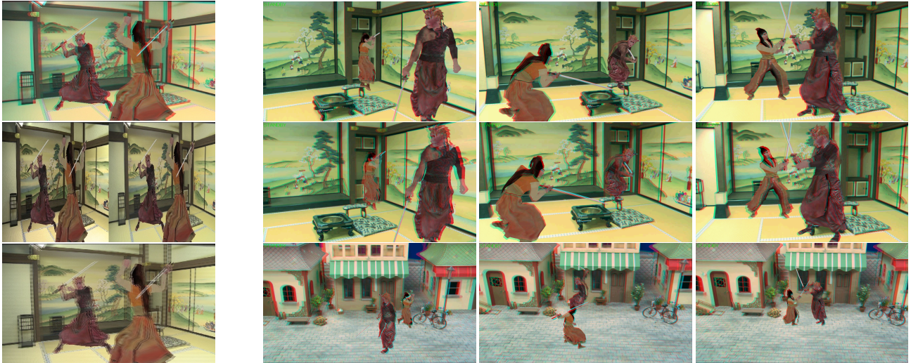
Figure 3: 3D format conversions and Figure 4: Examples of the Results of S3D MR-PreViz, Top and middle rows: Different setups in the switching, Top: Color anaglyph, Middle: same camerawork (Top: 6.0 cm of interaxial and 1.5 degrees of convergence, Middle: 6.0 cm of interaxial and 2.5 degrees of convergence), Bottom: On a miniature set using the same CGI data.
