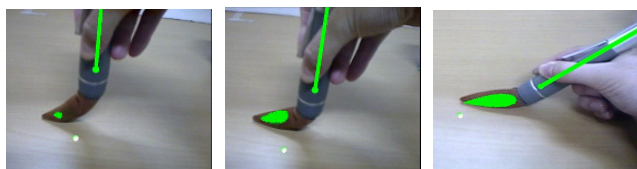
(a) しなり量・デバイスの傾きに応じた拡大・縮小 (a) Changing the shape of footprint depending on an amount of bending and tilt
