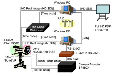
Figure 3 System configuration
