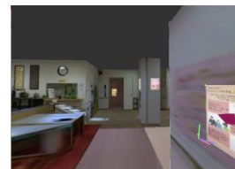
Part of the poster was out of camera view, which resulted in an inaccurate estimation of the camera position (22nd frame)
