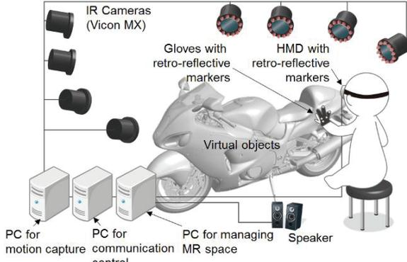
Figure 4: System configuration.
