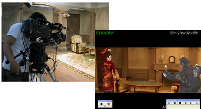
Fig. 2. Aspect of MR-PreViz image capturing and compositing system. (Left: Appearance, Right: Screenshot of composite images)
