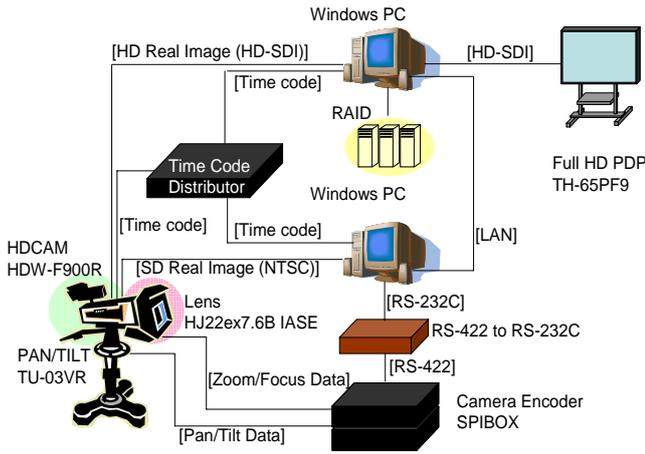
Fig.3. System configuration.
