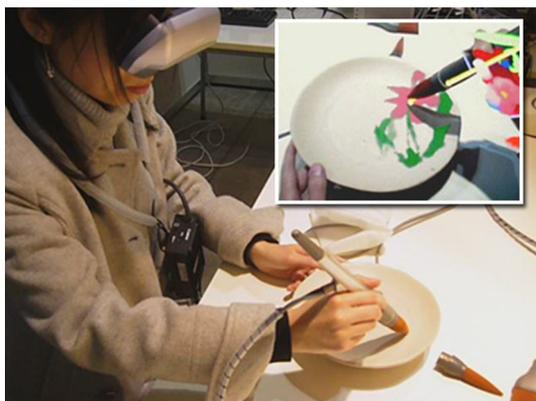
**Fig. 1** Using MAI Painting Expert 1.0 (Otsuki et al. 2010), a user paints with virtual ink directly on real objects
