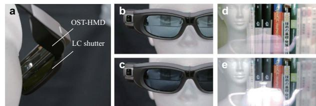
Figure 1: Our prototype OST-HMD (a-c) and conceptual images captured with a camera with automatic gain control (d, e). Our OST-HMD gradually reduces LC transparency (b to c) and increases the perceived brightness of the virtual content (Utah teapot) without making the user aware of real scene dimming (d to e).
