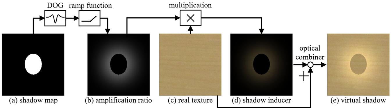
Figure 2: Data flow of the shadow inducer generation. (a) The shadow region is computed by the shadow mapping. (b) To calculate the ratio of the amplification, (a) is convolved with the DOG filter and cut of the negative. (c) Texture of the real scene can be taken from the user-perspective camera. (d) The shadow inducer is generated by multiplying (c) by (b). (e) Virtual shadow can presented by overlaying (d) on the real surface.
