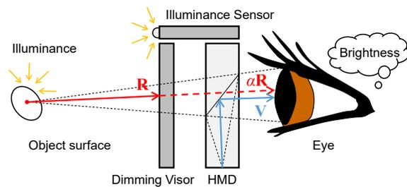
Figure 2: Schematic figure of the proposed OST-HMDs with dimming visors. The user receives the real light  $R$  through the unit angle  $\omega$ . While the virtual light  $V$  is directly projected to the eye by a display of HMD, the real light  $R$  is dimmed by the dimming visors to  $\alpha R$ .
