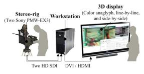
Fig. 3. System configuration
