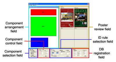
Fig. 5. Support tool for layout rule scheme
