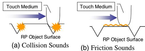
**Fig. 4.** Touch Sound Generated from RP Objects
